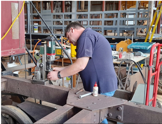
Trav redrills bolt holes in the chassis of Car 74
