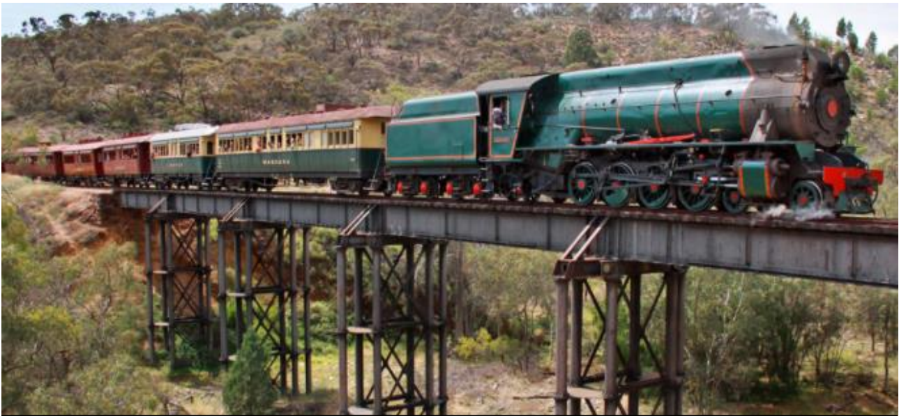
The Pichi Richi Railway's Locomotive W916 (ex-WAGR—Western Australian Government Railways). It's given the appearance of Broken Hill's Silverton Tramways Company's W22, which is also PRR's, but is at present out of service. It has some of W22's fittings such as the streamlined boiler top, and it carries W22's number. Shown here crossing the Woolshed Flat Bridge
