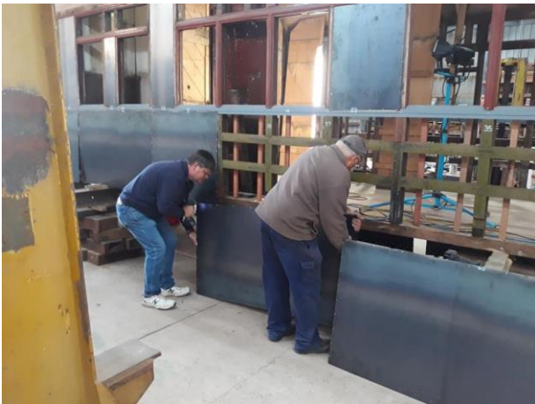
Fixing of sheeting to Car 470
