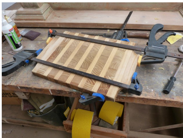
Small block chopping board reglued ready for oiling
