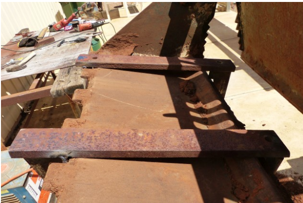
Quick fit ripper tynes fitted to bottom of loader bucket
