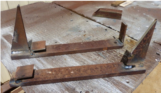
Dave constructed a set of quick fit ripper tynes for Kanga loader
