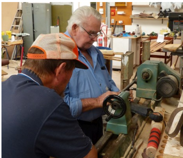
Andy and Col setting up guide rail on wood lathe
