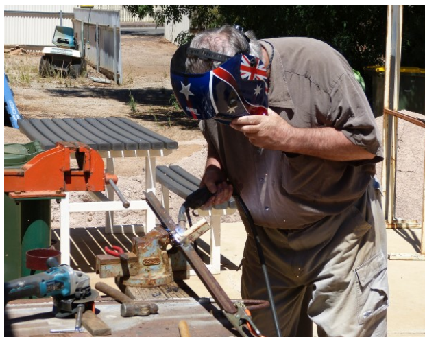
Rob making scraper gauge to set screenings level ready for pavers
