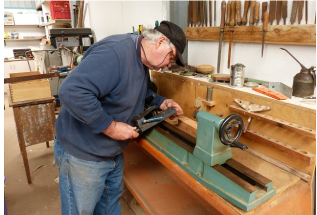
Rob setting up chisel rest on wood lathe
