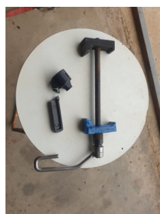
Repairs done to hold down bracket for wood lathe and easy tightener handle for chisel rest
